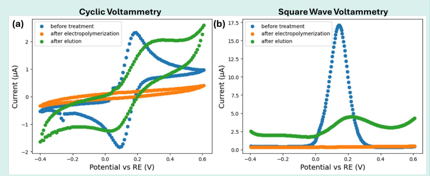
CV (left, cyclic voltammetry) and SWV (right, square wave voltammetry) measurements of the MIP formation on a CSPE (carbon screen printed electrode), performed in 2 mM Fc with 10 mM ammonia buffer pH 8.4.
