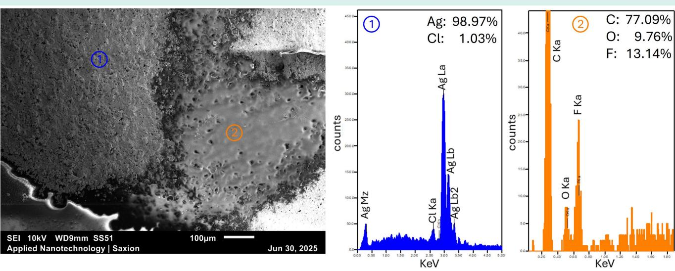
Left: SEM image of the Ag/AgCl counter electrode of a CSPE with a layer of PFOA. Right: Results of a SEM-EDS measurement on 2 different locations.
